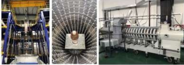
Klystron No. 1 Efficiency 65% (2020)
