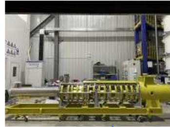
Klystron No. 2 Efficiency 77% (2021)
