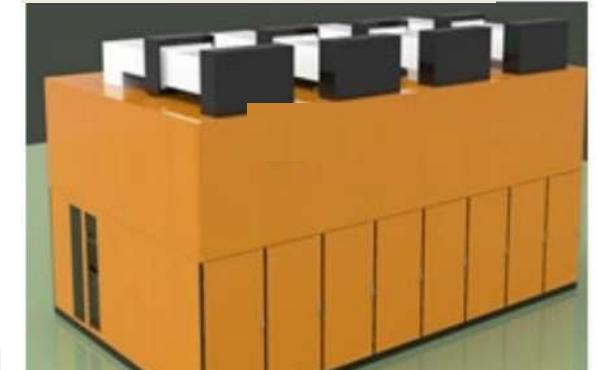
Klystron No. 3 (MBI) Efficiency 80.5% (under fabrication)
